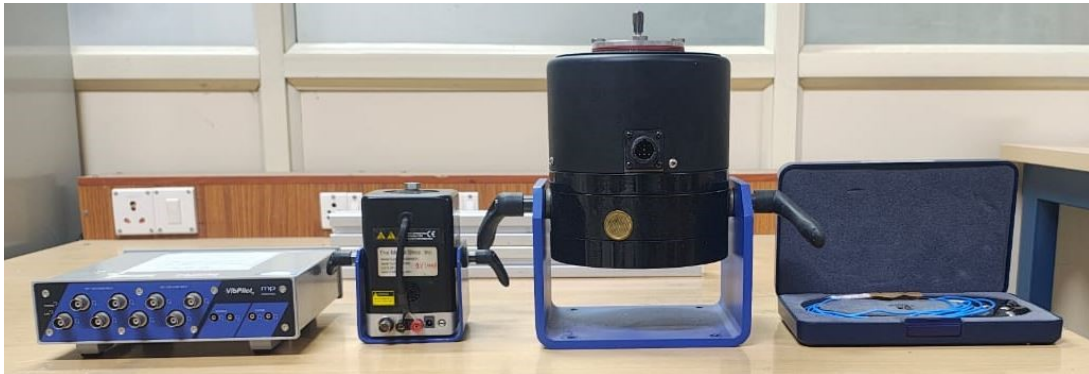
Figure 21: Modal Shaker with M+P Analyser with Triaxial Accelerometer.
