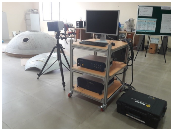
Figure 22: Laser Scanning Doppler Vibrometer from Polytec.
