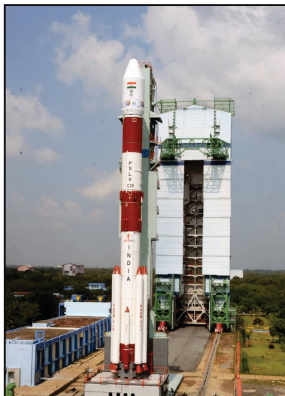
Photograph of PSLV-C25 , the rocket that carried Mars Orbiter Mission. The rocket has a height of 45 m, a diameter of 3 meters and weighs approximately 300 tonnes. The rocket can deliver payloads of up to 1500 kg weight into geosynchronous orbit. © ISRO
