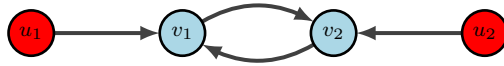
Figure 3.3: Networked system with two individual nodes and both nodes having external control input.
