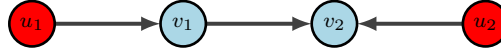
Figure 4.6: The networked system is controllable with parameters given in (4.10). Observe that there are no edge from node v_2 to node v_1 .
